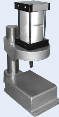
Column provides infinitely variable daylight settings and permits radial swing.
