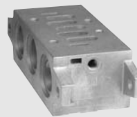
Modular element, one station ISO 5599/1, VDMA 24345 type C, bottom connections MI-013
